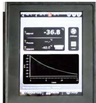
Sample temperature recording by optional immersion probe
