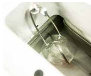
Sample holder in chamber (lid open)
