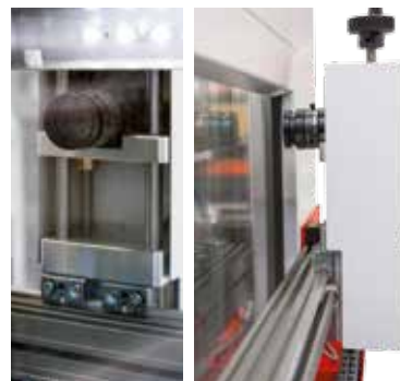
CCD Camera system for crack-growth measurement
