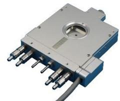
**HCS601G-IRM** FTIR heating and cooling stage with 24mm x 24mm sample area. Temperature Range -190°C to 600°C. Gas tight chamber with gas purge capabilities. CWD=10.5mm WD=10.5mm, cone angle>100°C. Includes IR windows. Offers a smaller temperature range than HS1200G, but supports LN2 cooling down to -190°C and a smaller footprint for better compatibility with optical instruments.
