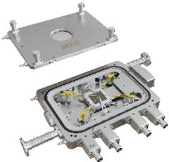
**HP1000G-PM** high-temp probing stage with 25mm x 25mm sample area. Temperature Range ambient to 1000°C. Gas tight chamber with gas purge capabilities. Includes four manual probe tips with coaxial BNC on the frame. Offers similar temperature control range and optical specifications to HS1200G, but also has integrated electrical probing capabilities.
