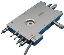
**HCS601GXY-IRM** FTIR heating and cooling stage with 24mm x 24mm sample area. Temperature Range -190°C to 600°C. Gas tight chamber with gas purge capabilities. CWD=10.5mm WD=10.5mm, cone angle>100°C. Includes IR windows. Has a wider temperature range, but a slightly smaller sample area, and is optimized for IR applications.
