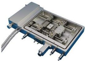
**HCS350G-TNS** heating and cooling stage for tensile force measurements. 26mm x 16mm sample area. Temperature range -190°C to 350°C. Gas tight chamber with gas purge capabilities. Apply up to 200 N force. Specialized for experiments requiring applied force control with simultaneous optical access.
