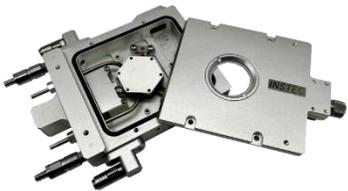
**HCP621G** heating and cooling plate with Ø28mm sample area. Temperature range -190°C to 600°C. Gas tight chamber with gas purge capabilities. Includes option to add electrical feedthroughs. Has a higher max temperature, but does not have a transmission aperture, and does not support evacuation. Highly compatible with reflection-mode optical instruments.
