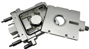
**HCP621G** heating and cooling plate with Ø28mm sample area. Temperature range -190°C to 600°C. Gas tight chamber with gas purge capabilities. Includes option to add electrical feedthroughs. Has a larger temperature range and more options, but does not support sample XY movement and does not have a transmission aperture. Highly compatible with reflection-mode optical instruments.
