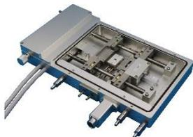
**HCS350G-TNS** heating and cooling stage for tensile force measurements. 26mm x 16mm sample area. Temperature range -190°C to 350°C. Gas tight chamber with gas purge capabilities. Apply up to 200 N force. Specialized for experiments requiring applied force control with simultaneous optical access.
