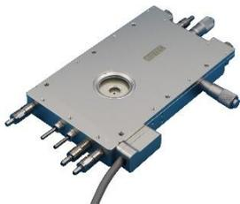
**HCS601GXY-IRM** FTIR heating and cooling stage with 24mm x 24mm sample area. Temperature Range -190°C to 600°C. Gas tight chamber with gas purge capabilities. CWD=10.5mm WD=10.5mm, cone angle>100°C. Includes IR windows. Has a slightly smaller sample area, but a larger temperature range and is optimized for IR applications.
