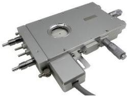
**HCS621GXY** heating and cooling stage with 28mm x 28mm sample area. Temperature range -190°C to 600°C. Gas-tight chamber with gas purge capabilities. Includes XY positioning and option to add electrical feedthroughs. Offers increased temperature range versus TSA12Gi, and also supports atmospheric control. Unlike TSA12Gi, requires LN2 for sample cooling, and is not designed for inverted microscopes.
