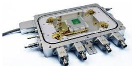
**TP102G-PM** heating and cooling plate with integrated electrical probers. 40mm x 40mm sample area. Temperature range -30°C to 120°C. Gas-tight chamber with gas purge capabilities. Perform optical analysis with simultaneous precision temperature control and electrical probing. Not designed for inverted microscopes.
