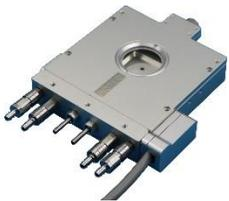
**HCS601G-IRM** FTIR heating and cooling stage with 24mm x 24mm sample area. Temperature Range -190°C to 600°C. Gas-tight chamber with gas purge capabilities. CWD=10.5mm WD=10.5mm, cone angle>100°C. Includes IR windows. Optimized for IR applications, and offers larger temperature range than TSA12Gi, but requires LN2. Not designed for inverted microscopes.
