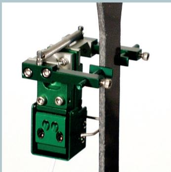
*Model 3475-050T-ST with  $\pm 0.050$  inch measuring range*
