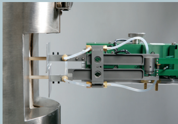
Model 3648 with 1 inch gauge length
