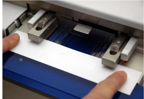
The test strip must not be touched in the test area
