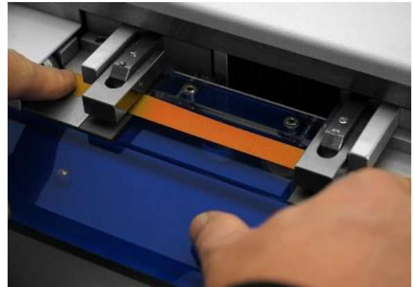
Insert a sample of width 15mm
